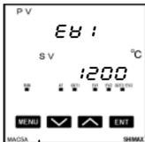
Initial value: upper limit absolute value measuring range Scaling upper limit lower limit absolute value measuring range Scaling lower limit
